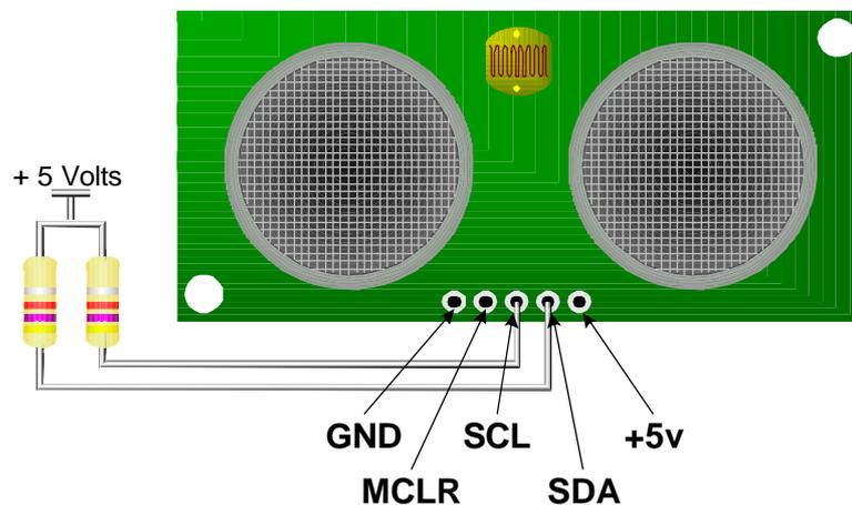
Ensure that a voltage of no more than 5 Volts is supplied to the SRF08, and that its polarity is observed, or damage 'will' occur.
