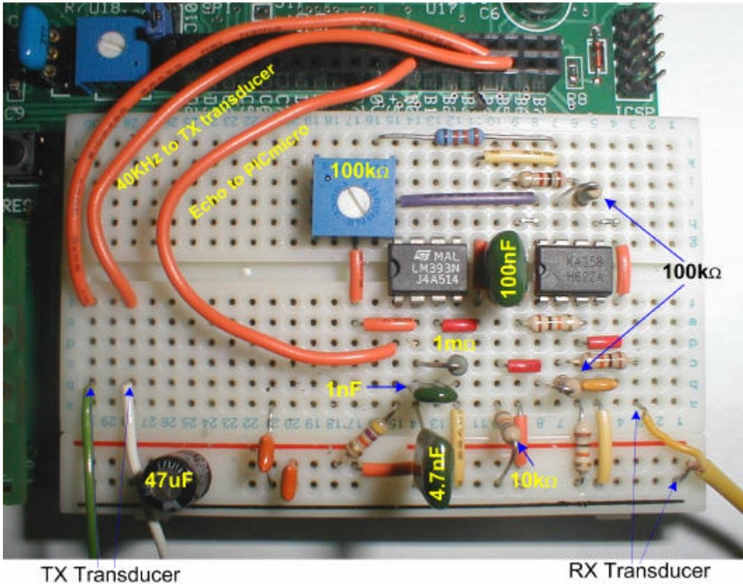
It's surprising what can be squeezed on to the small breadboard with a little care, the secret is the Wire Jumper kit also available from Crownhill. This offers both tidiness and repeatability as each wire length is colour coded differently. Anyway, a different angle photograph of the same board layout is shown below in order to clarify any obscured components in the picture above.
